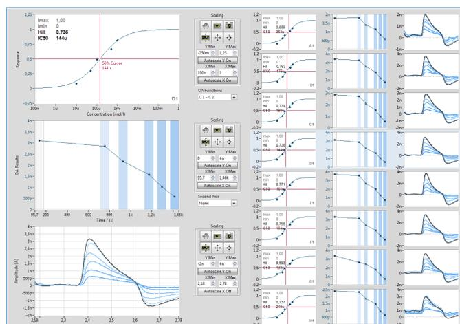
**Figure 3:** Screenshot of the analysis software, DataControl 96 showing inhibition of PepT1 by Lys[Z(No<sub>2</sub>)]-Val. 96 individual concentration-response curves were generated.
