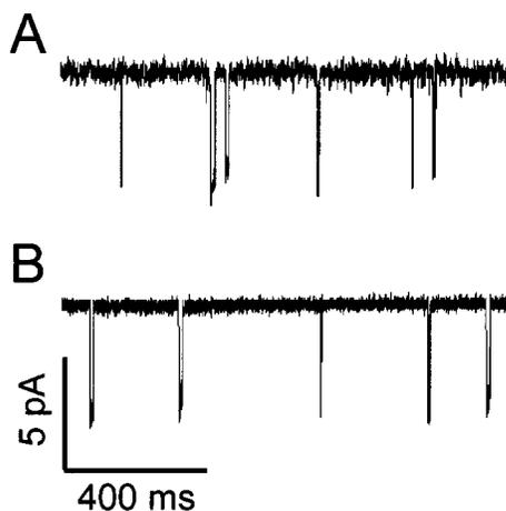
FIG. 2. Comparison of single channel currents recorded on the glass chip (a) and by the common glass pipette (b). Both recordings are performed on BK channels expressed in a mammalian cell line under identical recording situations, e.g., same solutions and amplifier settings, etc. The quality, e.g., time resolution and signal to noise ratio of data obtained can directly be compared.
