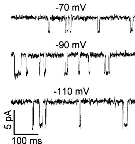
FIG. 3. Characterization of single ion channels using the glass chip: A BK-type  $\text{Ca}^{2+}$ -activated potassium channel is expressed in (CHO) cells (see Ref. 12) and single channels are recorded in a cell attached configuration at different holding potentials.
