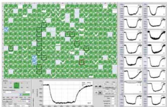
**Figure 5:  $\text{Kir2.1}$  endogenously expressed in RBL cells recorded on the SyncroPatch<sup>®</sup> 384PE.**  $\text{Kir2.1}$  was activated by addition of external solution containing high  $\text{K}^+$  concentration. Solution exchange rate is in the order of 50 ms on the SyncroPatch<sup>®</sup> 384PE.
