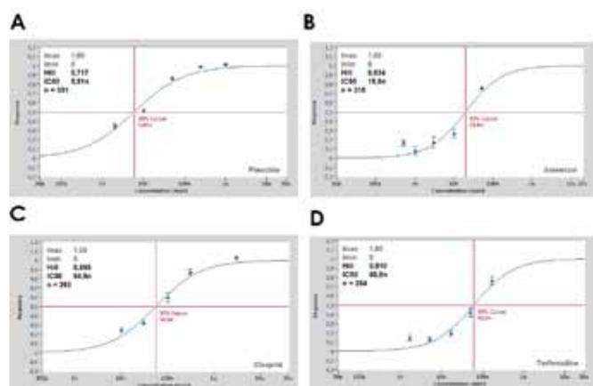
**Figure 2: Average concentration response curves for 4 different hERG blockers on the SyncroPatch® 384PE.** The concentration response curves were constructed across the whole plate (single concentration per cell). The SyncroPatch® 384PE analysis software (DataControl® 384) was used to calculate the average concentration response curves, normalized to maximum block and fitted with a standard Hill-equation. A summary of the IC<sub>50</sub> values and success rates is shown in Table 1.
